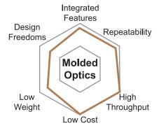
Regardless of optical molding technology, the reasons for selecting a molding process are similar: high-volume manufacturing, lower cost, repeatability, integrated features, and design freedoms.
