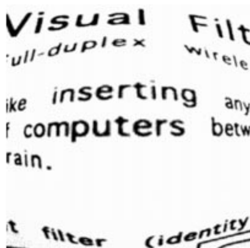
Figure 5. Using a visual filter such as this in the personal visual assistant may help a person with very poor vision to read. The central portion of the visual field is hyperfoveated for a high degree of magnification while allowing good peripheral vision.
