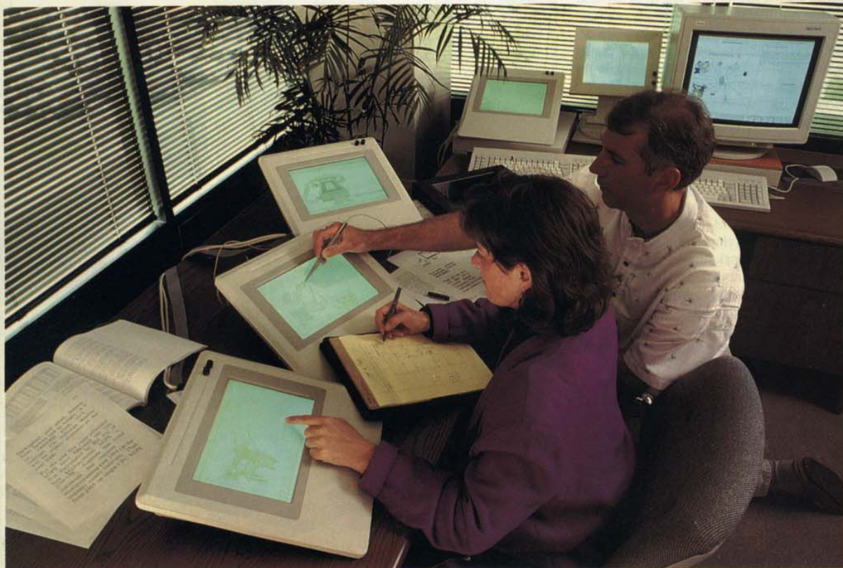
COMPUTER SCRATCHPADS augment the conventional screen in this office at the Xerox Palo Alto Research Center. Prototype pads are wired to conventional computers; thus far only a handful of wireless models have been built.
