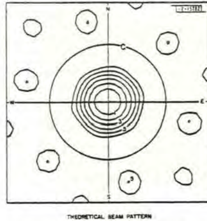
Fig. 28. Wavenumber impulse response of the array of Fig. 27.
