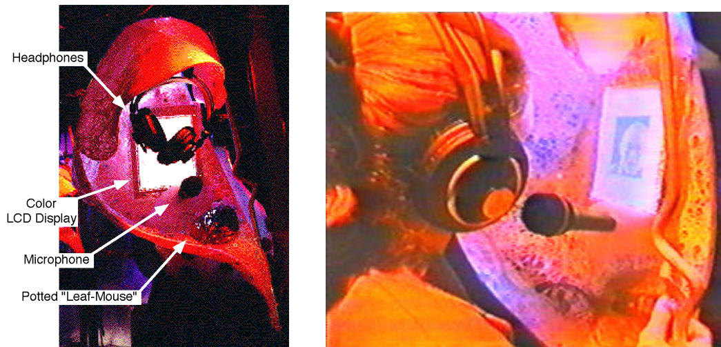
Figure 3: Layout and photograph of a Speaking Tree
