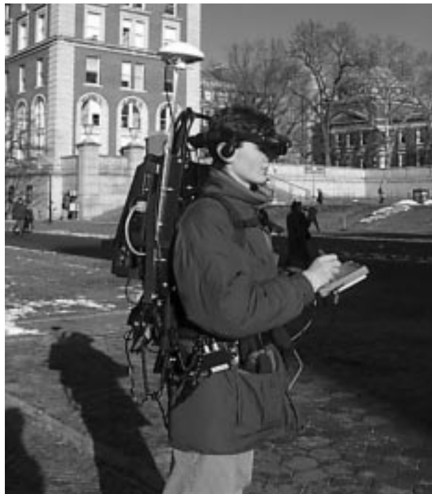
Figure 1. Prototype campus information system. The user wears a backpack and headworn display, and holds a handheld display and its stylus.
