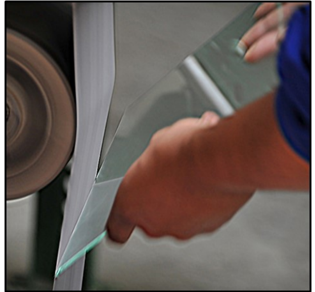
Seamed edge being produced via sanding belt to remove sharp edges
