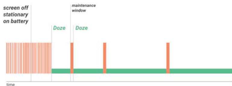
Figure 1. Doze provides a recurring maintenance window for apps to use the network and handle pending activities.
