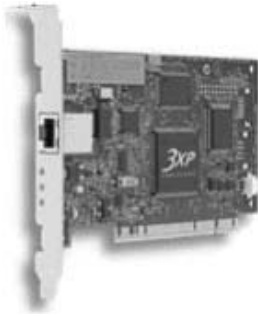
Figure 21: Network Interface Card with RJ45 connection.
