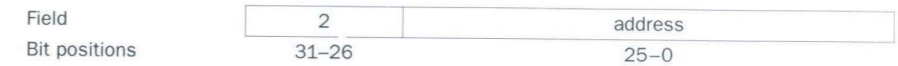
FIGURE 5.28 Instruction format for the jump instruction (opcode = 2). The destination address for a jump instruction is formed by concatenating the upper 4 bits of the current PC + 4 to the 26-bit address field in the jump instruction and adding 00 as the 2 low-order bits.
