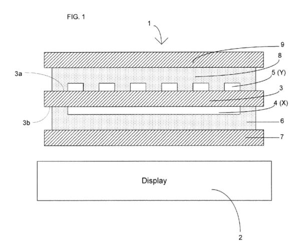
Figure 1 "is a cross-sectional view of an exemplary touch sensitive panel [(1)] and a display [(2)]." Ex. 1001, 2:3–4; *see also id.* at 2:52–53. The panel includes an insulating substrate 3 having two opposing faces, 3a and 3b. *Id.* at 2:53–61. Electrodes 4 (X) and 5 (Y), which may be arranged in different directions, are provided on faces 3b and 3a, respectively. *Id.* at 2:59–64.
