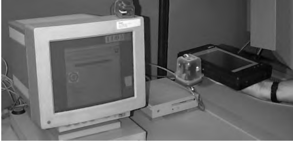
Figure 7. Home-made IR units allow cross-platform communication.
