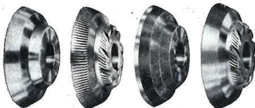
Fig 84-5. Types of rotors used in colloid mills. These may be smooth (for emulsification of most emulsions), serrated (for the emulsification of ointments and very viscous products), or of vitrified stone (for the emulsifications of paints and pigment dispersions) (courtesy, Tri-Homo).
