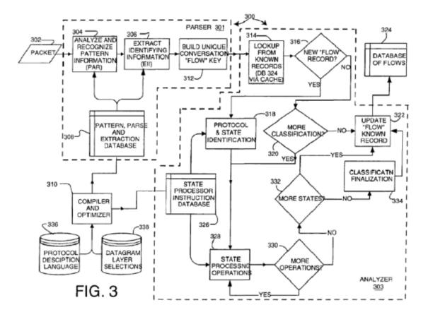
Figure 3 above shows network packet monitor 300. Id. at 8:48–13:50.
