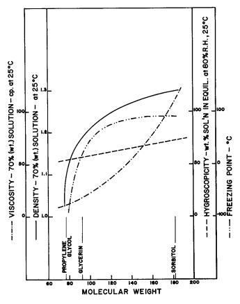
Fig. 1. Polyhydric alcohol behavior vs. molecular weight.
