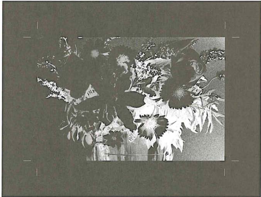
Simulation of a printed page with Negative and Emulsion Down options active
