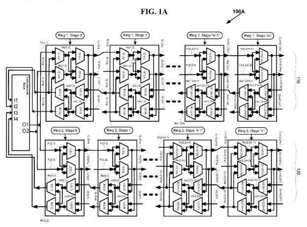
Figure 1A illustrates an exemplary partial multi-stage hierarchical network (or "block") in which each computational block has four inlet links I1, I2, I3, I4 and two outlet links O1, O2. *Id.* at 8:57–62. For each computational block, a corresponding partial multi-stage hierarchical network has two "rings" 110, 120. *Id.* at 8:62–9:3. Ring 110 has inlet links Ri(1,1), Ri(1,2) and outlet links Bo(1,1), Bo(1,2). *Id.* at 9:4–6. Ring 120 similarly has inlet
