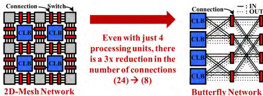
Figure 2: 2D-Mesh and Konda networks for a design consisting of 4 CLB blocks.
