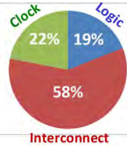
Figure 6: Power breakdown in a Virtex-5 FPGA.
