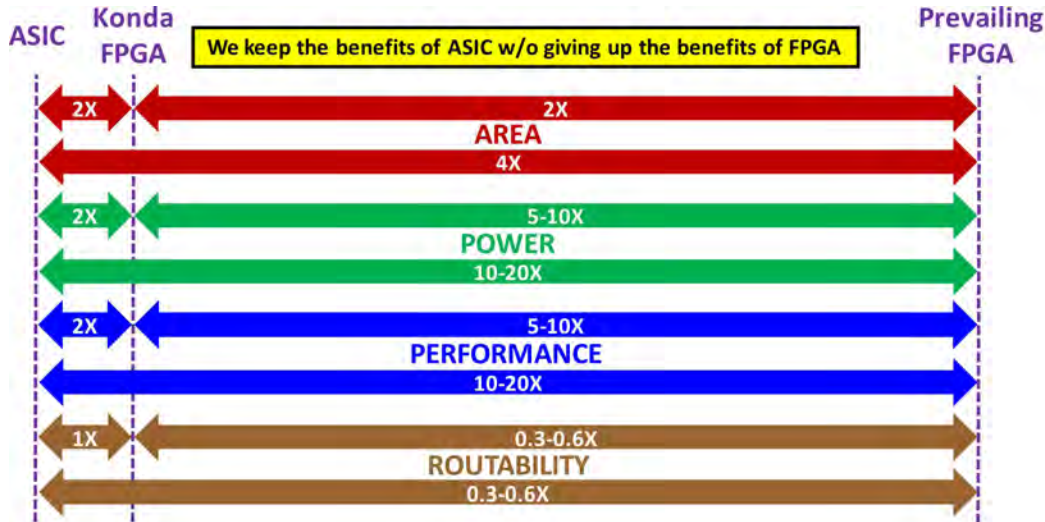
Figure 8: Konda interconnect network architecture has substantial benefits over today's FPGAs. It is projected to have ASIC-like energy efficiency, power, and performance. Such energy-efficiency levels are more than 100x better than general purpose processors.
