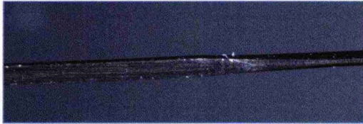
Guidezilla "crushed" substantially rigid portion
