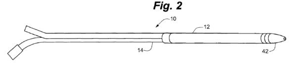
Figure 1 is a schematic depiction of a coaxial guide catheter and a tapered inner catheter and Figure 2 is a schematic depiction of these two elements assembled together. *Id.* at 5:40–45. As shown in Figure 1, coaxial guide catheter 12 includes tip portion 16, reinforced portion 18, and rigid portion 20. *Id.* at 6:34–35. Tapered inner catheter 14 includes tapered portion 46 at a distal end thereof and straight portion 48. *Id.* at 7:16–17. Clip 54
