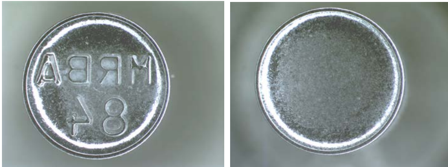
Figure 3 and 4. DL612 Upper Punches (Clinical Formulation with Avicel PH102)
