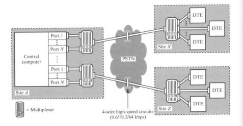
Figure 3.30 Multiplexer-based network schematic.
