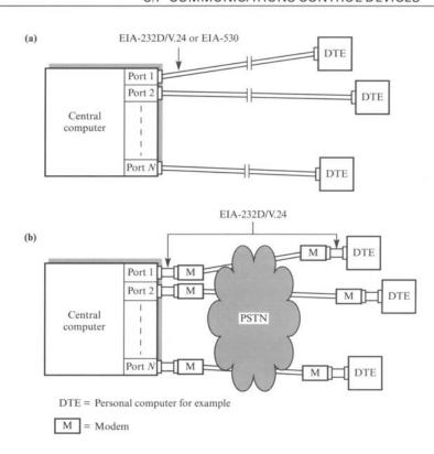
Simple terminal networks: (a) locally distributed; (b) remotely distributed.
