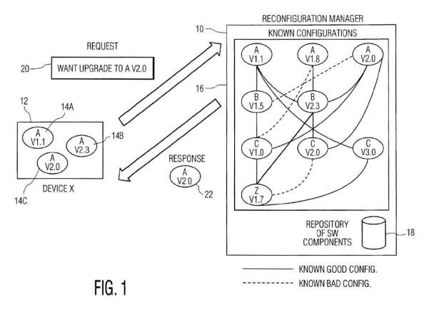
Figure 1 illustrates reconfiguration manager 10 interacting with electronic device 12, also referred to as "Device X." *Id.* at 3:14–16. When reconfiguration manager 10 receives a request for an upgrade from Device X, the request indicates that the device wants to upgrade to version 2.0 of software component A and includes a list of the components currently on the device, i.e., version 1.1 of component A, version 2.0 of
