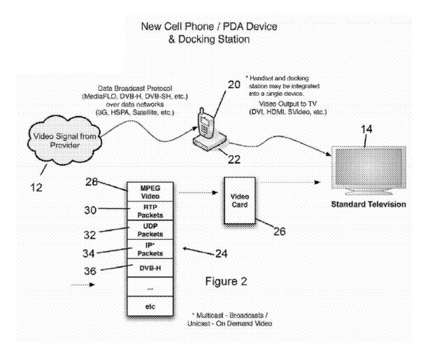
Figure 2, reproduced above, depicts mobile STB (10) facilitating the display in standard television (14) of data broadcast in unicast or multicast to mobile computing device (20). *Id.* at 4:47–51.
