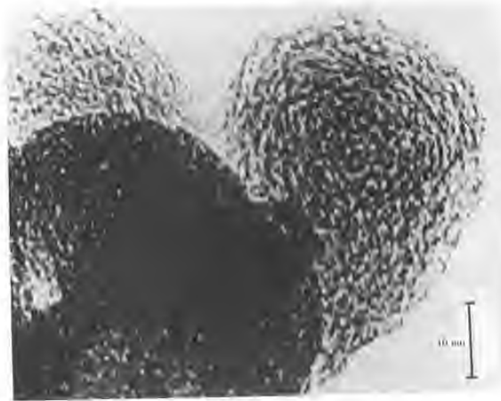
FIGURE 11-40 Lattice-imaging micrograph of a diesel particulate. 72
