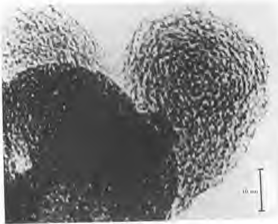
FIGURE 11-40 Lattice-imaging micrograph of a diesel particulate. 72
