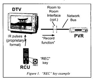
When the user presses the REC key, the RCU emits IR pulses in a proprietary format interpreted by the DTV receiver. The DTV recognizes the REC key is intended for whatever device the user has currently chosen as the
