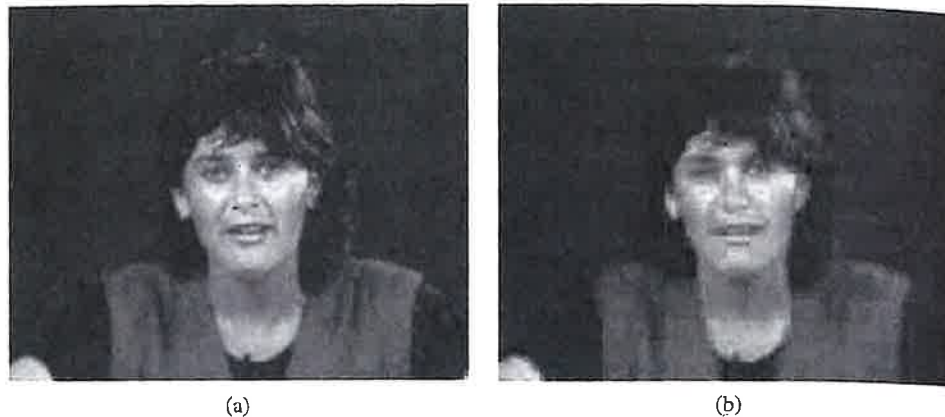
FIGURE 4 Severe blocking artifacts introduced by gross quantization of DCT coefficients: (a) original, (b) reconstructed. (See color section, p. C-27.)
