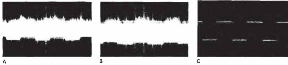
Figure 9.36. Scope photos showing excellent noise immunity of differential data transmission (75108 differential receiver). (Courtesy of Texas Instruments, Inc., Dallas, Texas.) A. (+) receiver input. B. (-) receiver input. C. Receiver output.
