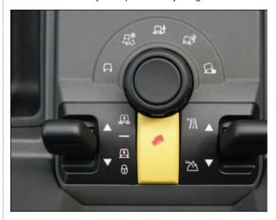
First introduced on the Discovery 3 and now fitted as standard on the Rar Rover Sport, it optimises driveability and comfort whilst maximising tractic is simple to operate via a rotary switch on the centre console with five terr settings.
