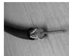
Figure 12: RG-8 coaxial cable.
