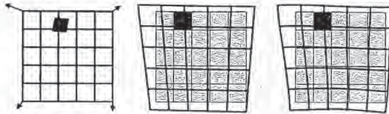
Fig. 2. We exaggerate here the distortion applied by StirMark to still pictures. The first drawing corresponds to the original picture; the others show the picture after StirMark has been applied – without and with bending and randomisation.
