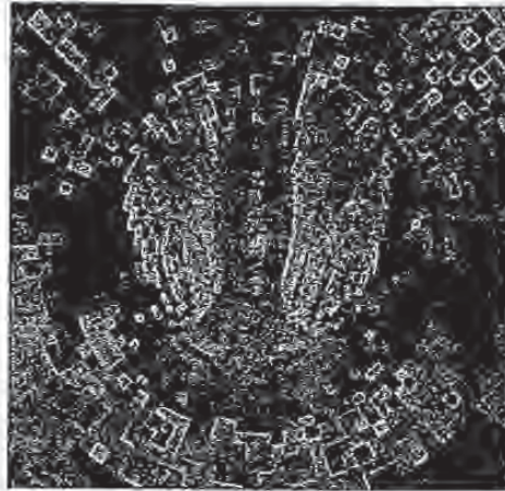
Fig. 7. The image of a mandrill reconstructed from a log polar map of size 100 \times 100 samples. This reconstruction uses nearest neighbour interpolation.
