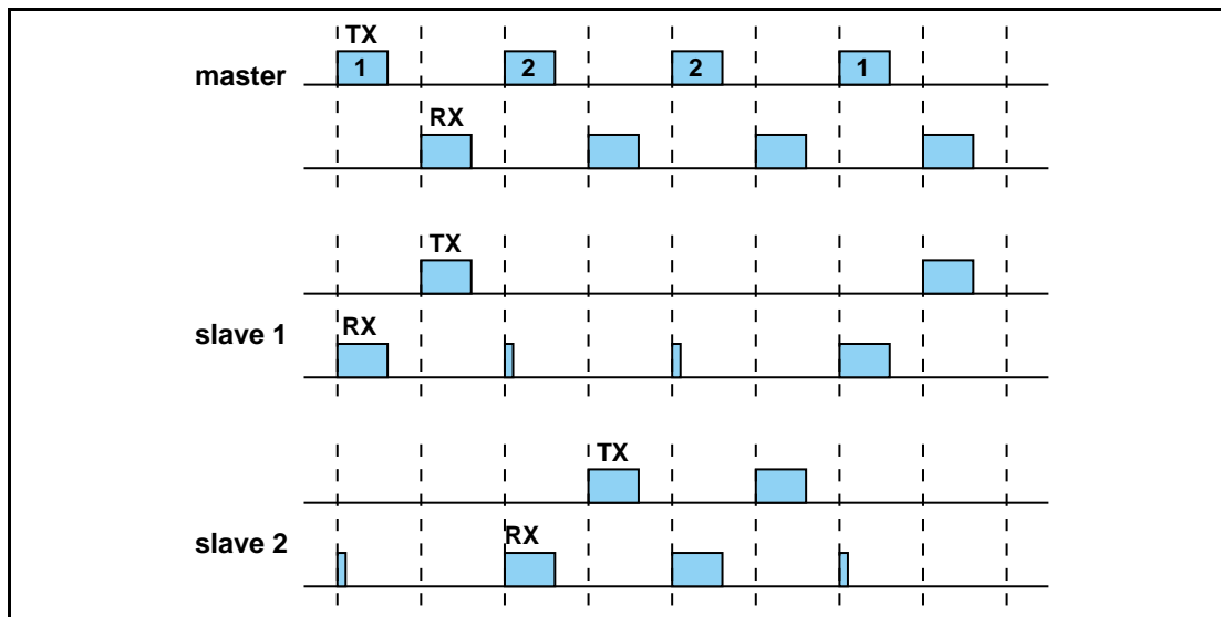
Figure 8.6: RX/TX timing in multi-slave configuration
