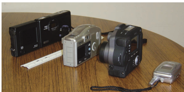
Figure 1. Cameras from 1995 through 2003. As technology improved, cameras became physically smaller, shrinking display size accordingly.
