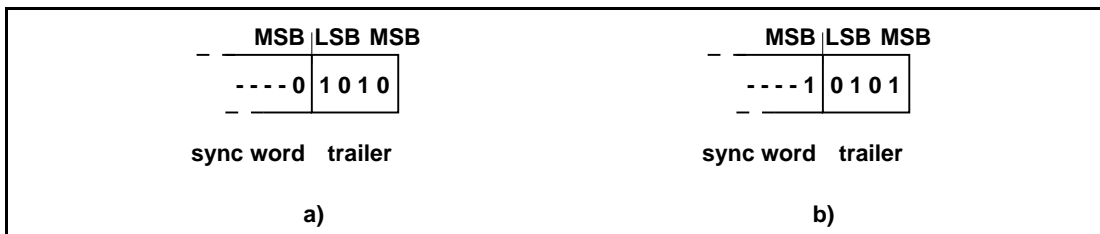
Figure 6.7: Trailer in CAC when MSB of sync word is 0 (a), and when MSB of sync word is 1 (b).
