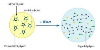
In presence of water, SEPINEO™ P 600 reverses and the polymer network deploys instantly, forming a perfectly stable gel in a few seconds.
