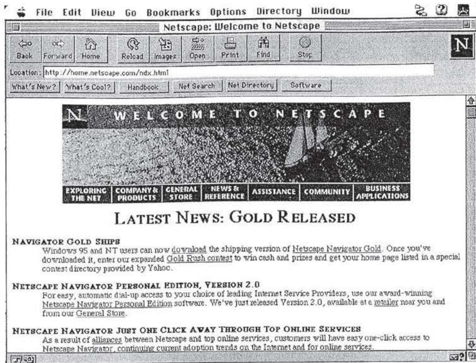
FIGURE 1.7: Netscape Navigator for the Mac works almost exactly the same way as the PC (and for that matter, Unix) version of the program, except for the normal Macintosh user-interface features, such as the menu bar being at the top of the screen instead of below the title bar.
