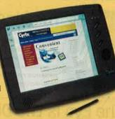
NO WIRES: The Cyrix WebPad. and accesses the Internet wirelessly via a radio-frequency base station-a set-top box or standalone base station.
