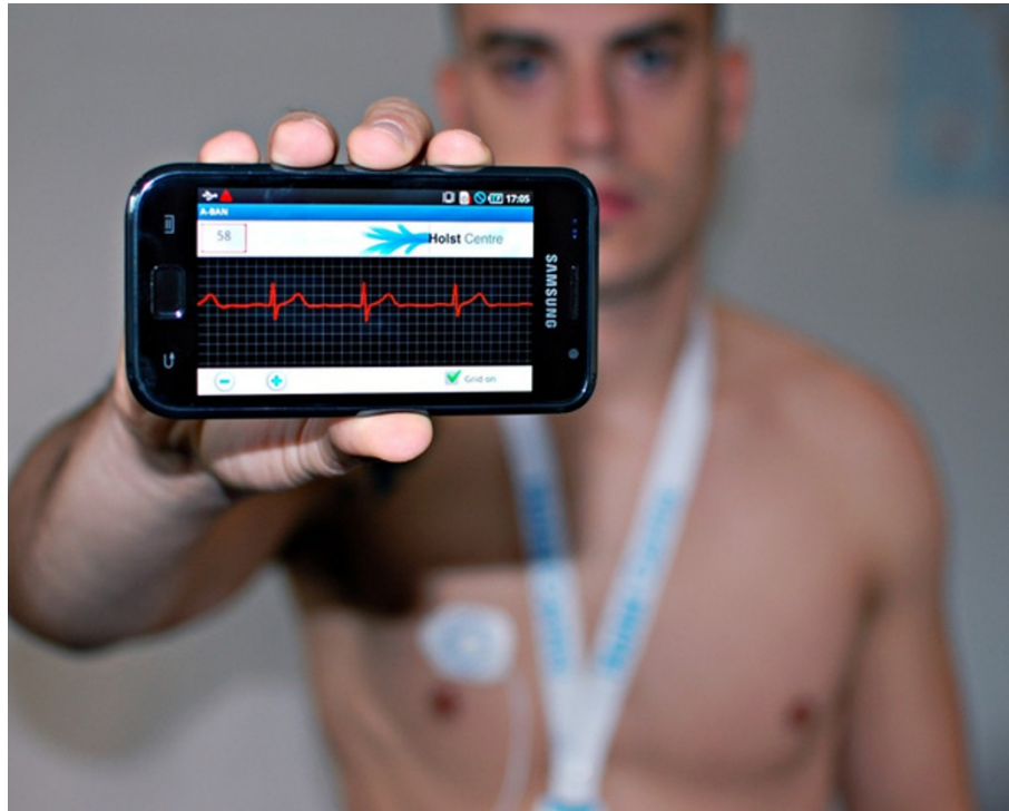
Figure 4 Smart phone based ECG monitoring system by IMEC. The Android based mobile application allows low power ECG sensors to communicate wirelessly with the phone. With increasing computational and storage capacity and ubiquitous connectivity, smart phones are expected to truly enable continuous health monitoring. (Courtesy of IMEC, The Netherlands).
