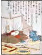
Copper beating pictorial record in the Kodo Zuroku (Source: Sumitomo Historical Archives)
