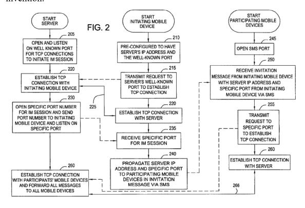
In Figure 2, the initiating device transmits a request 215 to establish a connection with a server. *Id.* at 4:55–59. Once the connection between the server and initiating device is established 220, the server transmits a port number to the initiating mobile device, which receives the port number 235,
