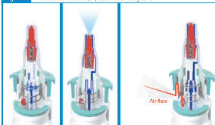
Figure 3: Function of a mechanical preservative-free system.
