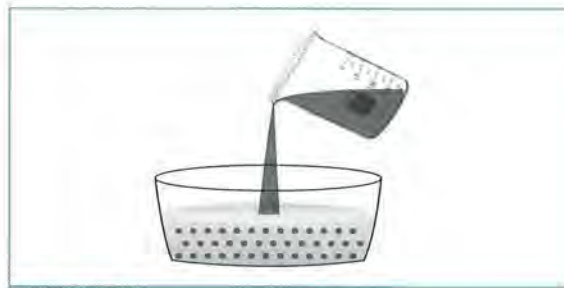
FIGURE 1-20. The volume of a tank can be determined from the amount of substance added and the resulting concentration.
