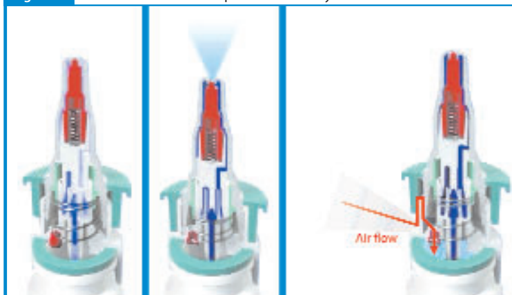
Figure 3: Function of a mechanical preservative-free system.
