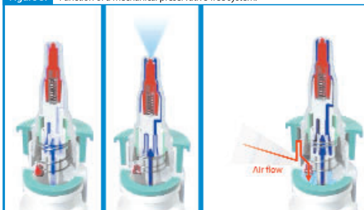
Figure 3: Function of a mechanical preservative-free system.
