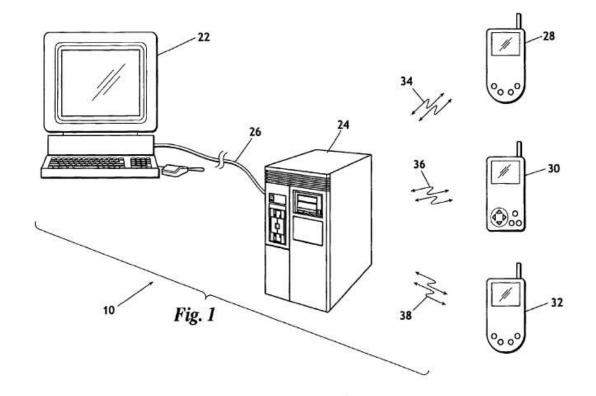
In particular, Figure 1 shows system 10 including server 24; handheld computers 28, 30, and 32, which are operated remotely from server 24; and computer 22, which provides for administration of the system and reviewing data collected by the system. *Id.* at 7:13–23, Fig. 1. Server 24 is connected to computer 22 via Internet 26, a local area network, or a private wide area
