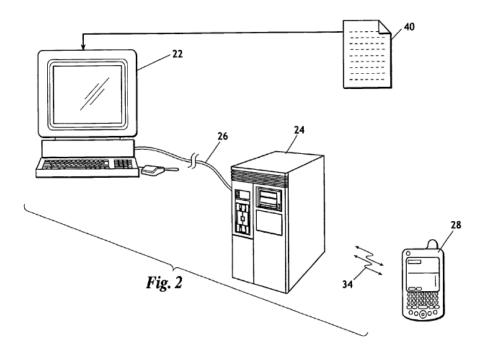
Figure 2 shows system 10 is used to create questionnaire 40. Ex. 1001, 8:38–9:6. Computer 22 has an interface that allows a user to create this questionnaire and distribute it to handheld devices. *Id.* at 8:38–50. As the client enters questions and selects response types, server 24 builds a stack of questions and responses, and assigns indices, or tokens, which point to each question or response. *Id.* at 8:53–56, 9:3–6. Each token can correspond to a
