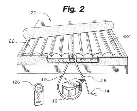
Figure 2 shows an air mattress system comprising pump 112, left and right air hoses 116 and 118, left and right bladders 122 and 124 of inflatable bed 120, and controller 126. *Id.* at 3:61–4:10. Pump 112 has an air inlet, an air outlet, and a processor board that receives signals from controller 126 to increase or decrease pressure in left bladder 122 or right bladder 124. *Id.* at 4:3–6, 10–15.
